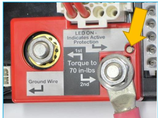
(2.7) Turn on Main Power Switch and verify that the LED illuminates.
