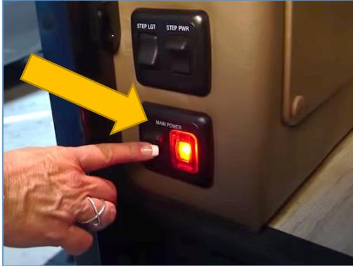
(2.1) Power off system by turning the Main Power Switch to the off position (located just inside the entry door).
