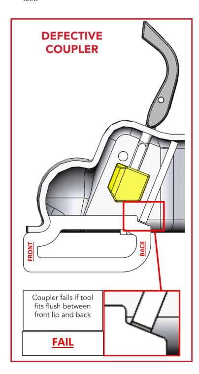
**Step 2 -** Insert the tool into the ball socket. Make sure the front of the tool is being pressed firmly into the lip of the coupler.
