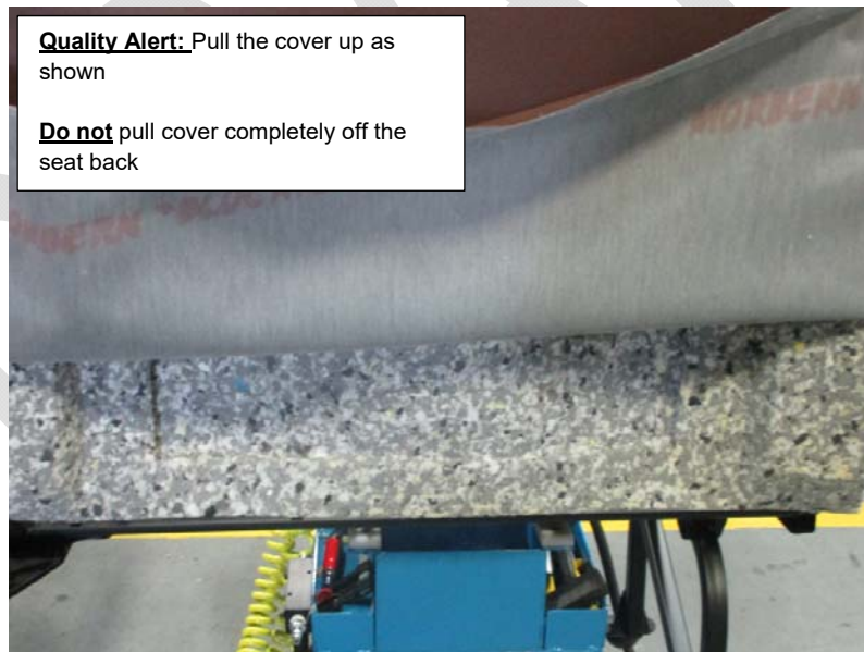
Figure 5 : Pull up the cover (back of seat)
