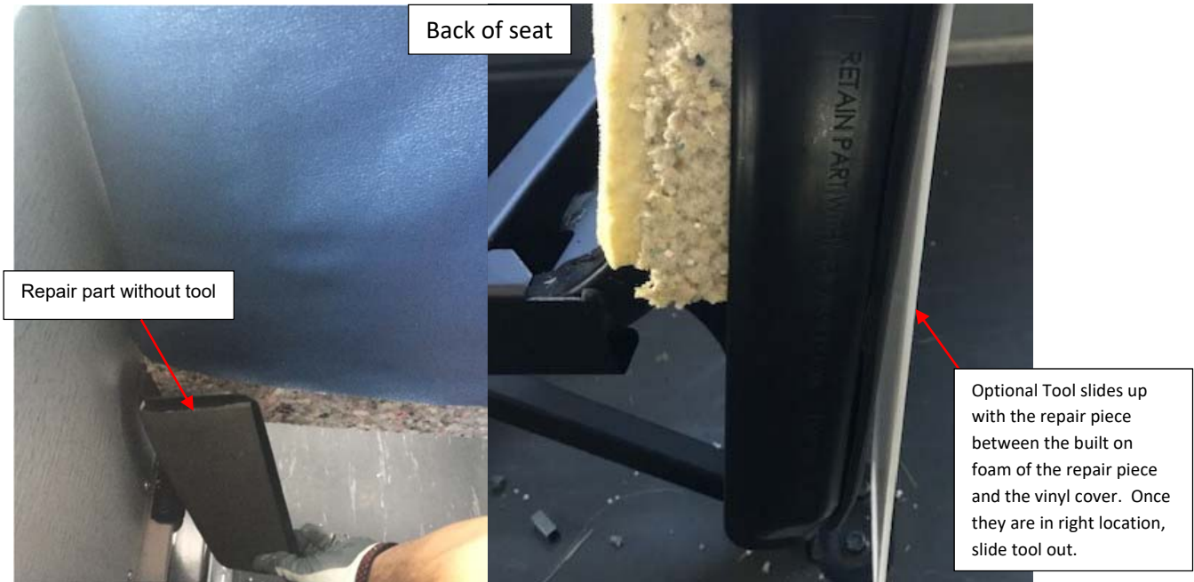
Figure 6: Positioning the Repair part in place ( standard on Left and with available tool on right)
