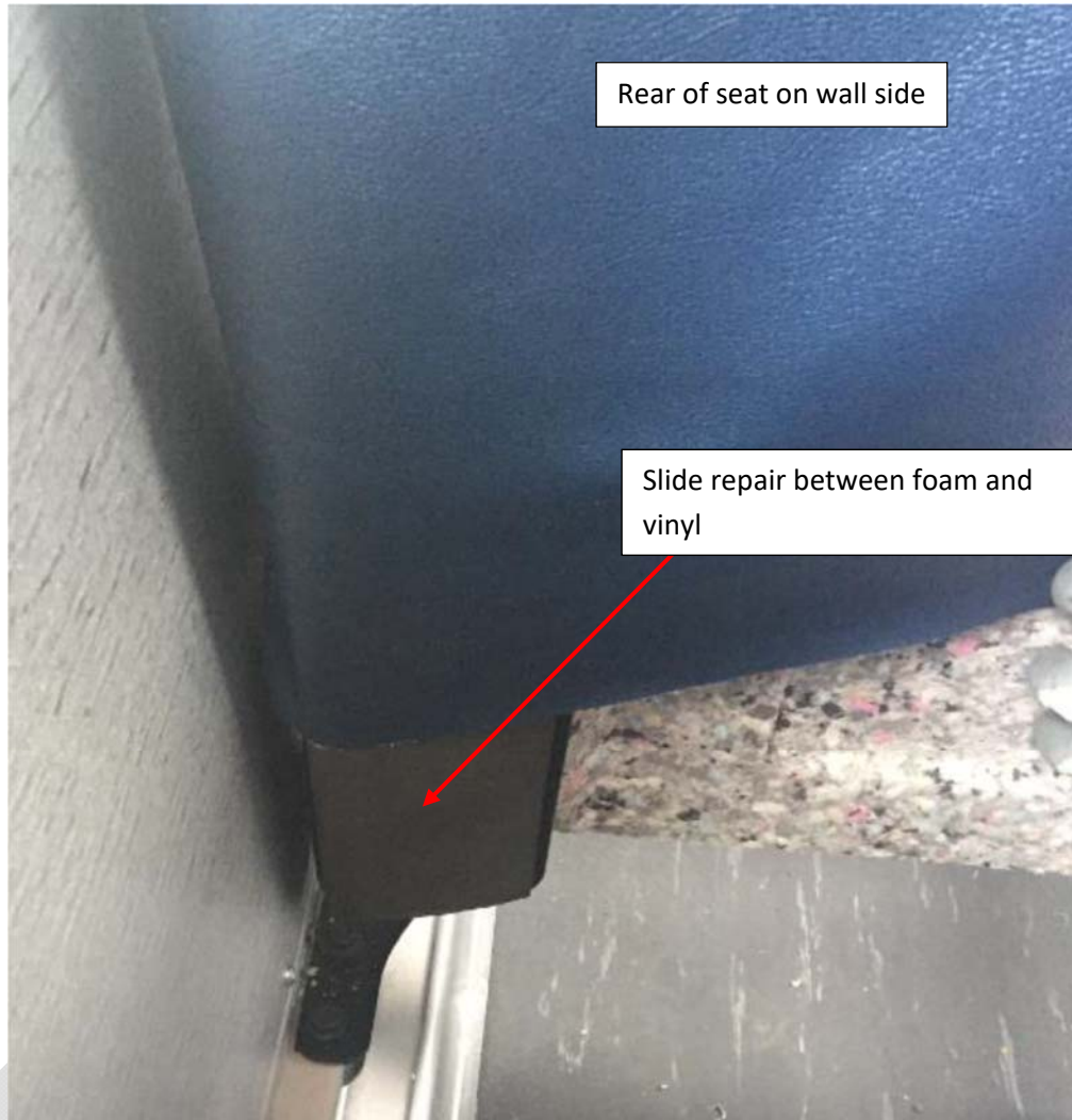
Figure 7: Seat shown with repair part inserted
