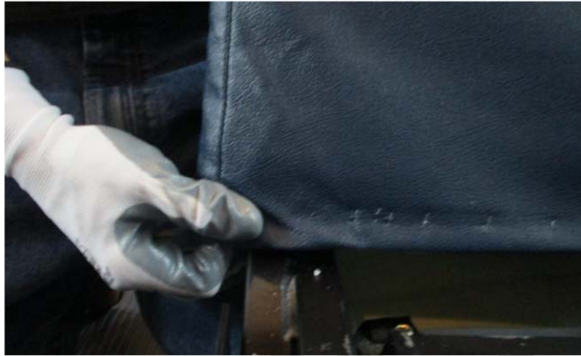
Figure 12: Showing how the Vinyl will look when folded and stapled
