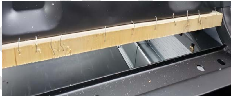
Figure 3: Staples bent over wood piece using pliers
