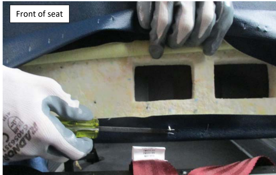
Figure 2: Removal the staples from the back side of the vinyl
