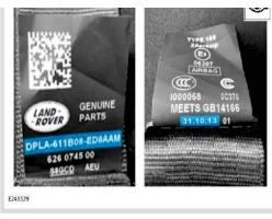
Vehicles with ebony seatbelts only: inspect both sides of the front left seatbelt label for the production date and part number.
