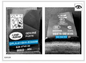
Vehicles with espresso seatbelts only: visually inspect both sides of the front left seatbelt label for the production date and part number.
