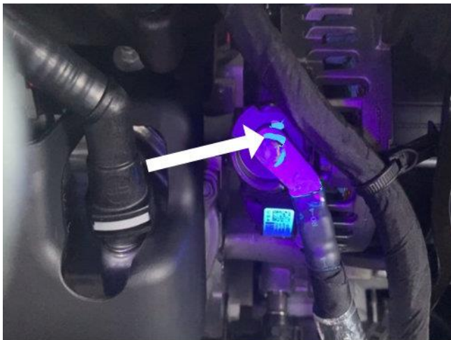
Unacceptable Glue Contamination (Black Light Image)
