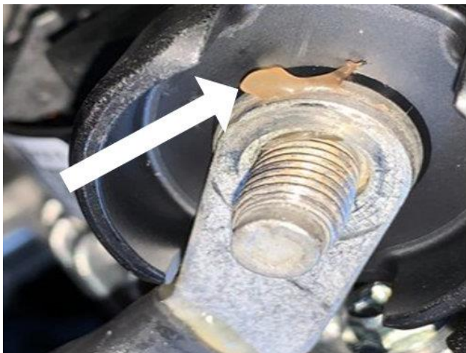
Unacceptable Glue Contamination (Daylight Image)
