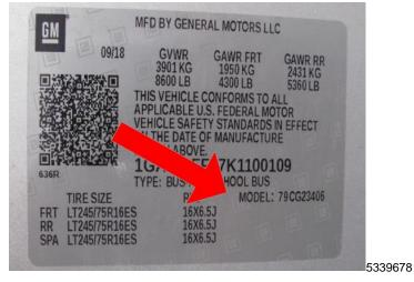
**NOTE**: Locate the model number on the information label positioned in the lower rear area of the driver door (example shown above only - see the correct model numbers for short and long wheel base model numbers below).
