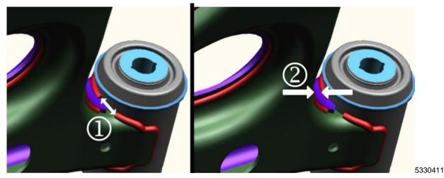
Photograph of Gap 1 (between the welds, red) and Gap 2 (between the control arm body and bushing barrel, purple).
