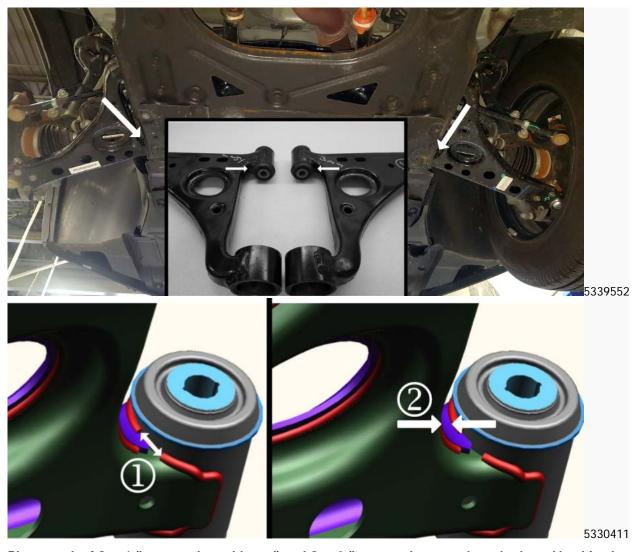
Photograph of Gap 1 (between the welds, red) and Gap 2 (between the control arm body and bushing barrel, purple).
