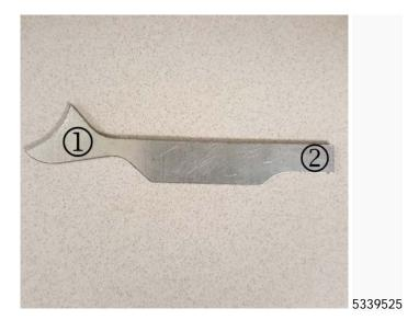
Photograph of the Inspection Gauge. Use the gauge to measure two weld gaps on the lower control arm. Use the number one (1) side of the gauge to measure the weld gap in step 4 and the number two (2) side of the gauge to measure the weld gap in step 5.
