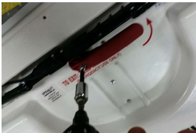
Step 13: The inside of the red handle has ribs to self-orient the red handle on the outer handle.
