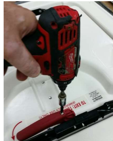
Step 6: Insert the 1/8" Allen bit into the 008798 screw and remove screw from red handle.
