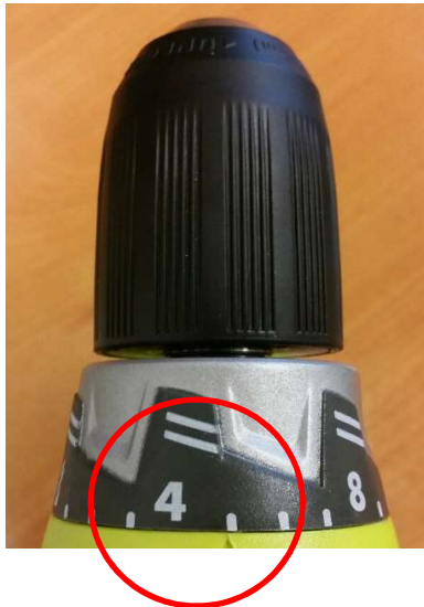
Step 5: Set the torque setting to 4-5, or the minimum needed to set the screw.
