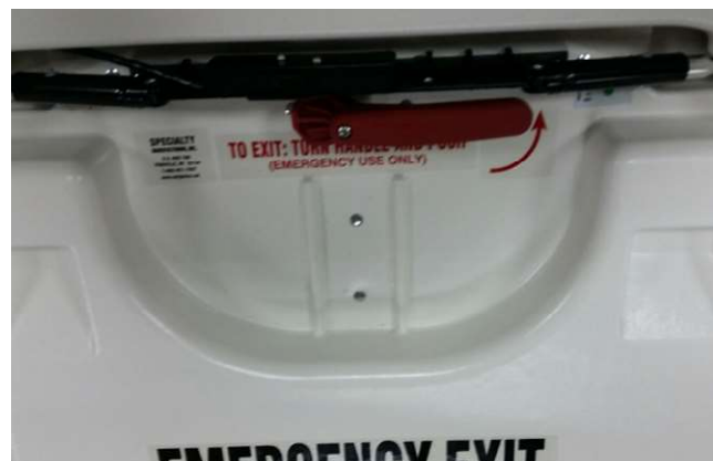
Step 4: REWORKING THE HATCH Rotate the handle into the orientation shown
