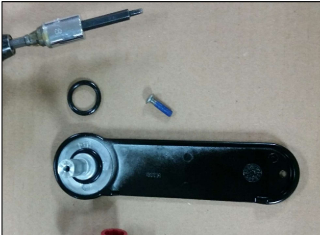
Step 1: Gather the necessary components for the work. 009336 Handle, 009321-5 O-ring, 008798 Screw, 1/8" Allen wrench or driver w/ 1/8" bit
