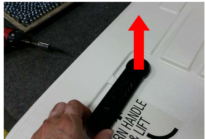
Step 8: Open the lid 5-6 inches, reach around and lift the black handle out of the bushing.
