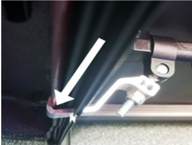
Correct installation of bracket clamp hook
