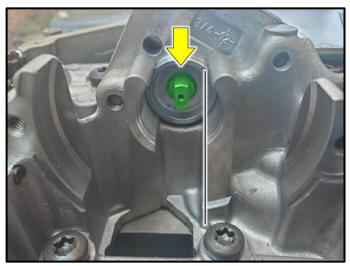
Turn the pump shaft <arrow> in a vertical orientation as shown.
