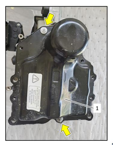
Temporarily reinstall cover <1> with bolts <arrows>. This will prevent contamination of the mechatronic.
