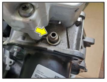
The mechatronic is filled through vent pipe <arrow> with 1.1 L of hydraulic fluid.
