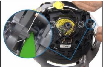
Apply removal wedge -3409- between horn ring and inflator <1> and press together locking elements using longnose pliers <2>. Lever off horn ring at plastic lugs <3>.
