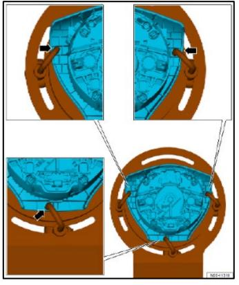
Clamp airbag centrally in airbag support. There are securing points on the sides <arrows>, parallel, opposite each other, and below.
