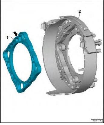
Included in the replacement parts kit is an insert ring <1>. This must be used when installing a new inflator and placed in the horn ring <2>.
