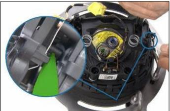
Apply removal wedge -3409- between horn ring and inflator <1> and press together locking elements using longnose pliers <2>. Lever off horn ring at plastic lugs <3>.
