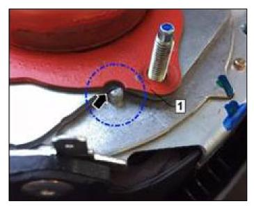
Install the new inflator onto the studs.
