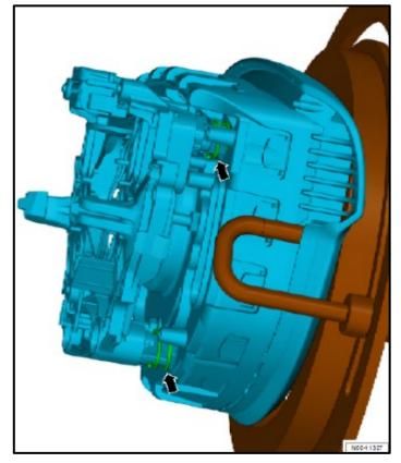
Fit springs <arrows> for horn ring again if necessary.
