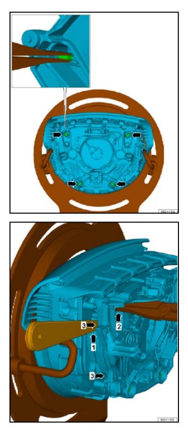
• Remove locking pins <arrows> for horn ring with aid of longnose pliers.
