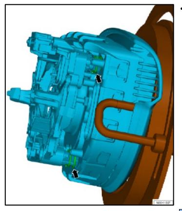
Position horn ring with springs on securing clips and press firmly in place. Ensure that springs are seated correctly on both sides <arrows>.
