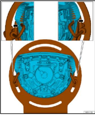
Clamp airbag centrally in airbag support. Securing points on the sides <arrows> and parallel opposite each other.
