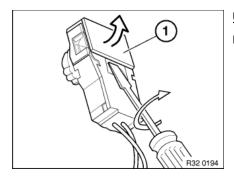
Unlocking the airbag plug connection:
