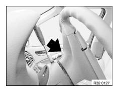
Release screws (Torx T30) on both sides.
