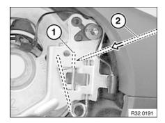
Use the screwdriver (2) to press on the lock (1).
