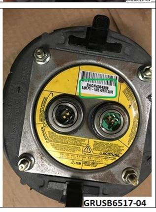
Some vehicles may have air bag control unit MRS III which was introduced in some models starting September 1999 and supports a dual stage gas generator
