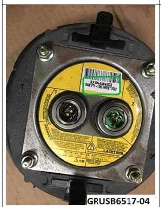
**Situation 3:** Some vehicles may have air bag control unit MRS III which was introduced in some models starting September 1999 and supports a dual stage gas generator.
