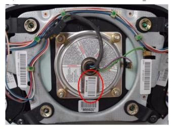
parts label(s) on the gas generator on the back.
