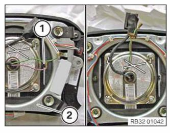
• Release both the connectors (1) on the airbag unit (2).
