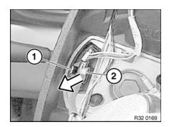
Press down lock (1) and disconnect plug (2).
