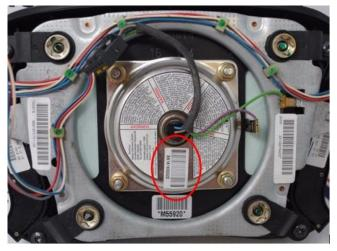
Once the air bag is removed and the wiring is disconnected, turn the air bag over to read the parts label(s) on the back.
