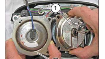
Remove the previous gas generator (1) and subsequently directly place the new gas generator (2).
