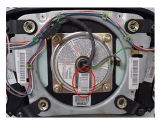
Once the air bag is removed and the wiring is disconnected, turn the air bag over to read the parts label(s) on the gas generator on the back.
