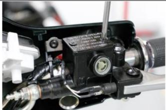
Connect one end of a transparent tube to the bleed nipple, placing the other end of the tube into a suitable container.
