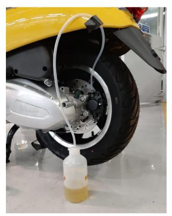
This will ensure that all the fluid in the brake circuit is replaced correctly with new fluid.
