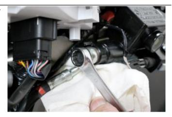
Fit the bleeding kit fitting with bleed nipple, P/N AP8133945 with new copper washers, P/N AP8113004, and loosen the bleed nipple nut to open.
