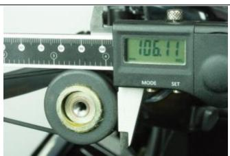
Once the distance between the lever and the hand grip is correct, replace the brake fluid with the following procedure.
