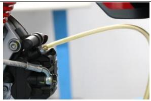
Bleed the front caliper from the bleed nipple with the procedure described below:
