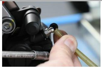
Fit the O-ring P/N **006731**, as shown in the figure. **Note: O-ring found in kit 1R000467**
