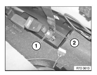
Seat belt is coded against incorrect installation.
