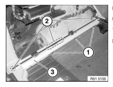
Release clamps (1). Unfasten screws (2). Tightening torque 51 47 15AZ. Feed out lashing rail (3) to the front. BMW Group - AIR: 2019-11-25 / 09:56 Retailer: -/-Model: X5 xDrive40e iPerformance Development code: F15 Model code: KT03 Lead type: KT03
