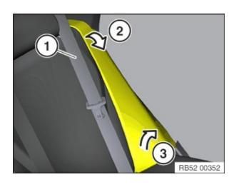
Pull seat belt (1) to middle and place behind head restraint.
