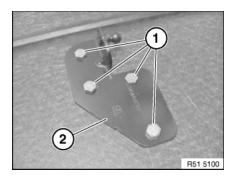
Push retaining spring (1) to end of gas pressure spring.
