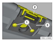
Release screws (1). Remove cover (2) and retaining hook (3). BMW Group - AIR: 2019-11-25 / 09:58 Retailer: -/-Model: X5 xDrive40e iPerformance Development code: F15 Model code: KT03 Lead type: KT03
