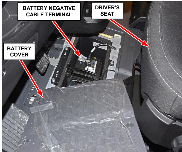
Figure 1 – Battery Cover and Negative Cable
