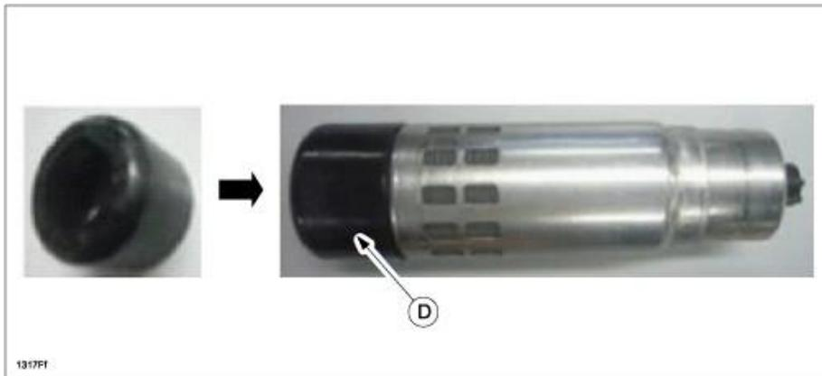
b. Insert the new inflator and align the side of the retainer and guide line of the inflator (A).
