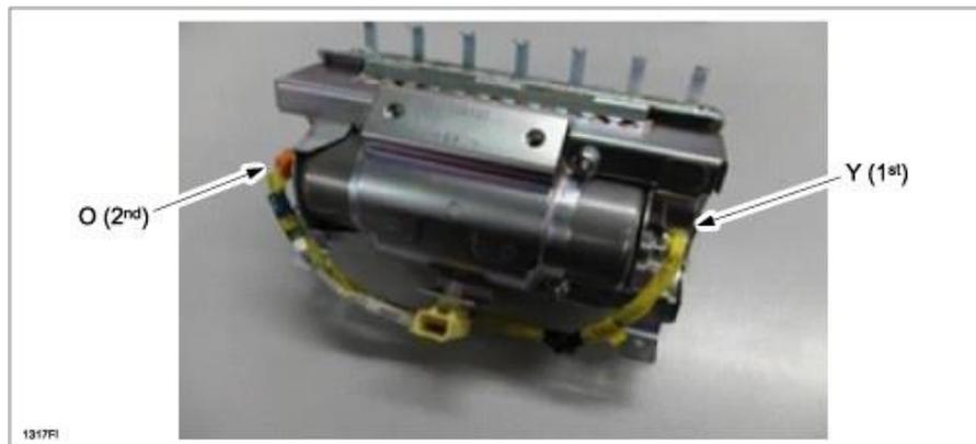
1. Remove the connector of the harness assembly.
