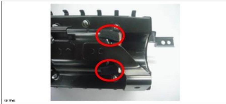
6. Insert the new inflator into the retainer
