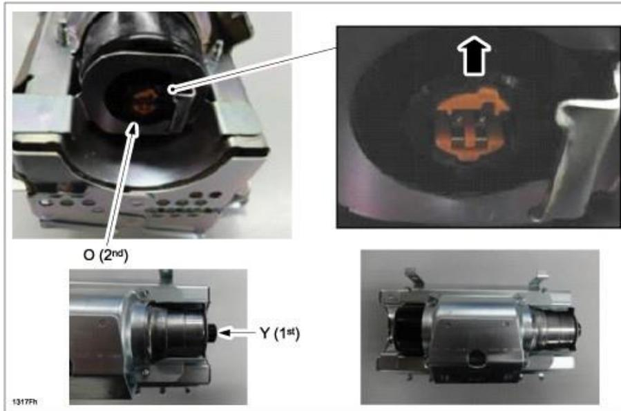
6. Install the new stopper to the retainer.
