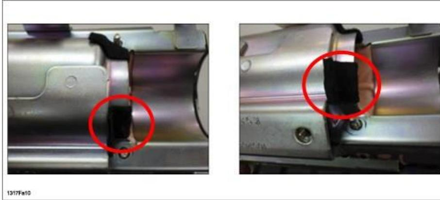
5. Insert the new inflator into the retainer
