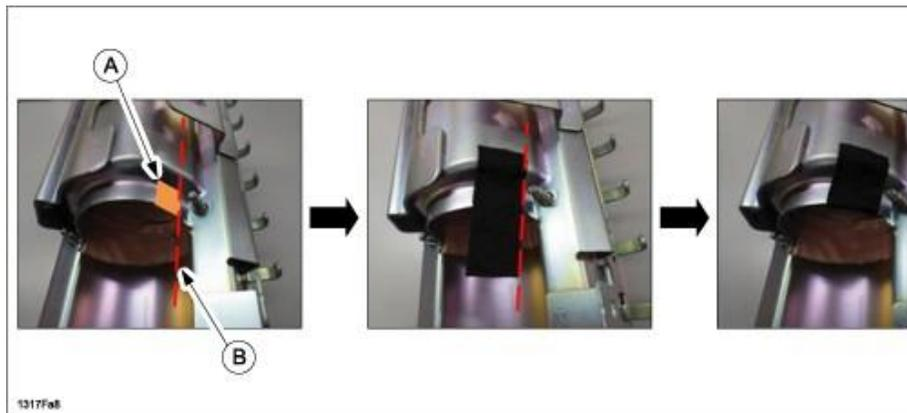
b. Attach the other felt tape on the other side of the retainer.
