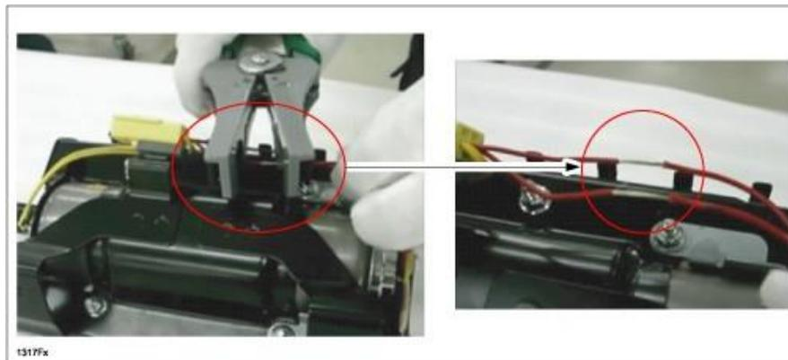
c. Connect the two wires by twisting them together (for both wire harnesses).
