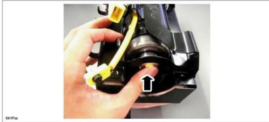
5. Attach the felt tape (A) to the retainer in 2 places.
