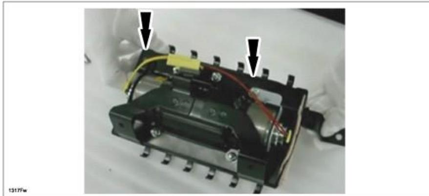
b. Strip the insulation from the two wires as shown.
