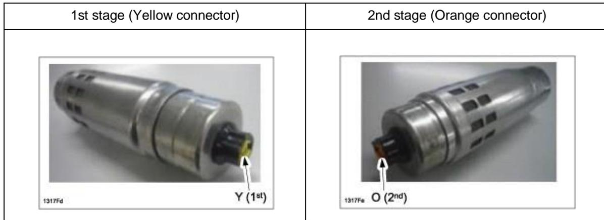
a. Attach the collar D to the 2nd stage side of the new inflator.
