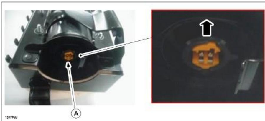
8. Install the new stopper to the retainer.
