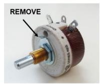
Connect the Pot1 wire (smaller terminal) to the potentiometer center tab (carefully bent the center tab 45deg).
