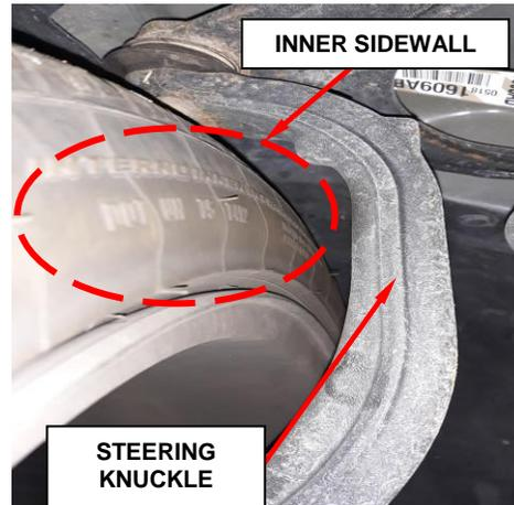
Figure 1 – Tire Inner Sidewall
