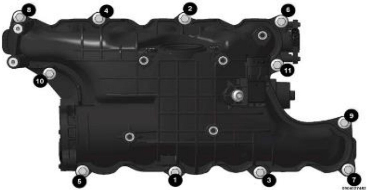
Figure 28 – Intake Bolts Tightening Sequence
