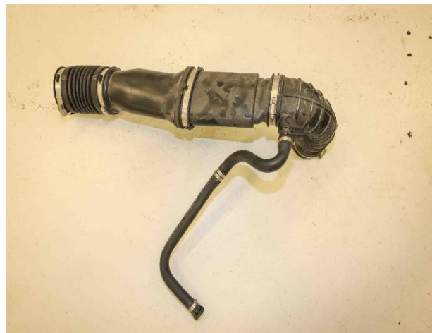
Figure 33 – Intake Air Tube Assembly
