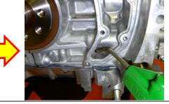
**CAREFULLY** blow air into the oil pan-side passage to collect the remaining PCV valve components.
