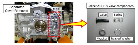
**TIP:** If any PCV valve components remain in the oil pan-side passage, **CAREFULLY** apply compressed air to the oil pan-side passage as shown below.
