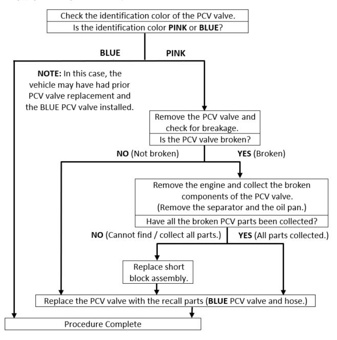
**STEP 1:** Locate the PCV valve and check the identification color. If for some reason the color cannot be identified, remove the PCV valve and confirm the condition (failed / come apart). If the (unidentifiable) PCV valve is not broken, replace it with a new (**BLUE**) valve and PCV hose. If the valve is broken, proceed as if it were a **PINK** valve using the flow chart(s) above as a guide.
