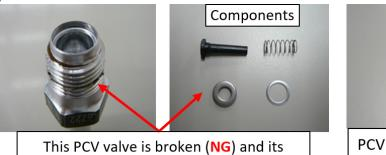
This PCV valve is broken (NG) and its components have fallen into the engine.
