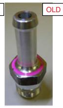
NOTE: P.n. SOA635322 (ThreeBond 1217H) is to be used for the PCV valve thread sealer.
