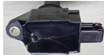
Cracks and Fissure
