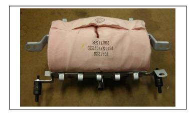
e) Mount the adaptors (579943-3R3) to the airbag as shown.NOTE: The 6mm stud mounts to the airbag.
