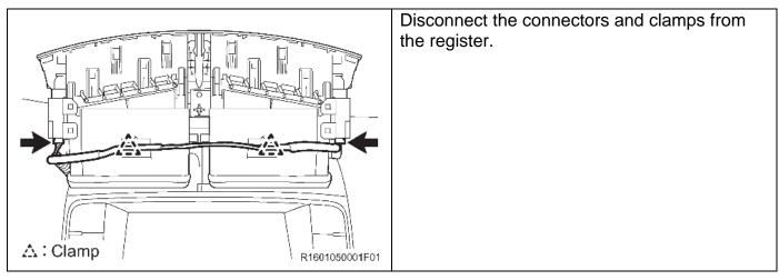
NOTE: DO NOT contact the postioning tabs while removing the instrument panel as the panel could be damaged.
