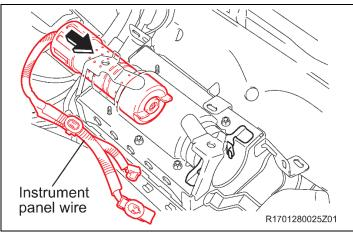
1. **INSTALL THE NEW INFLATOR** a) Install the new inflator as shown.
