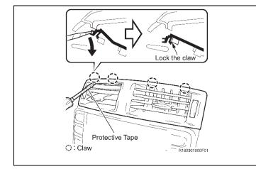
Removing the No. 3 air register
