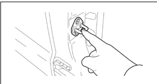
If the anti-static kit is not available, before starting work and periodically while working on the vehicle, touch a metallic part of the vehicle to discharge static electricity in the body.
