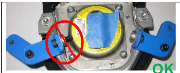
**NOTE: Ensure that the bolts that attach the bracket to the airbag DO NOT protrude past the threaded portion of the horn mounting ring.**
