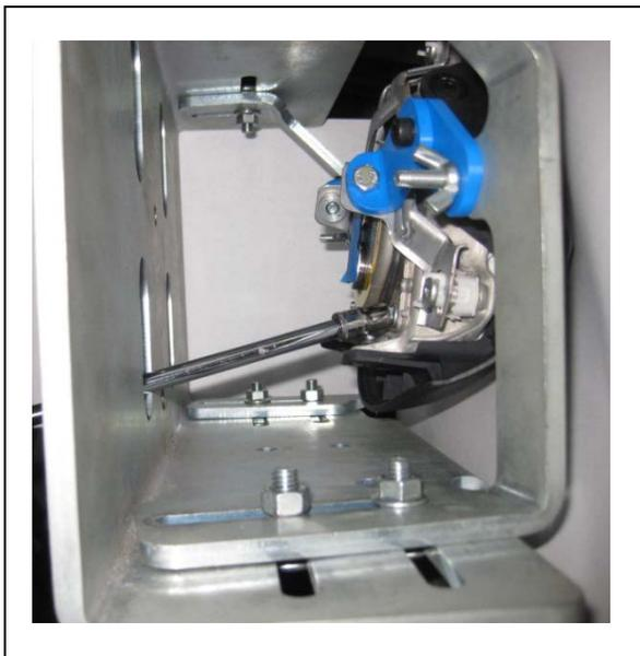
**6. REMOVE THE SELF LOCKING NUTS**
