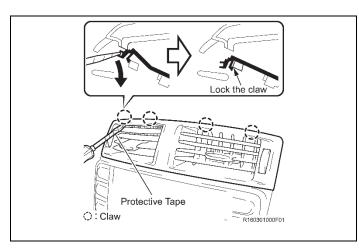
Removing the No. 3 air register
