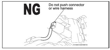
NOTE: When removing the register DO NOT push on the connector or wiring as it could be damaged.
