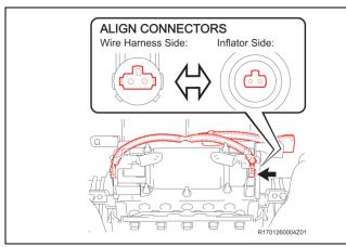
Connect the connector and the secondary lock
