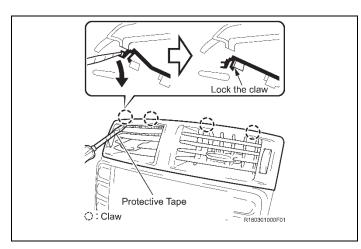
Removing the No. 3 air register
