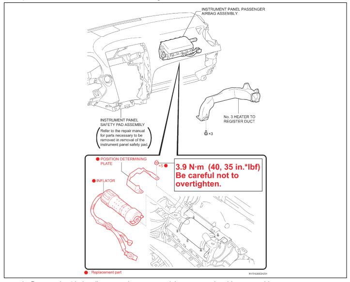
c) Remove the 4 bolts, disengage the straps, and then remove the airbag assembly.
