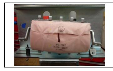
f) Mount the airbag to the mouting bracket as shown.
