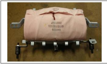
e) Mount the adaptors (579943-3R3) to the airbag as shown.
