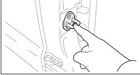
Before starting work and periodically while working on the vehicle, touch a metallic part of the vehicle to discharge static electricity in the body.
