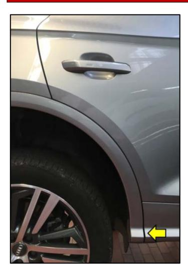
Replace clips for lower wheel arch trim "cap" <arrow> on both left rear and right rear wheel arch trim.
