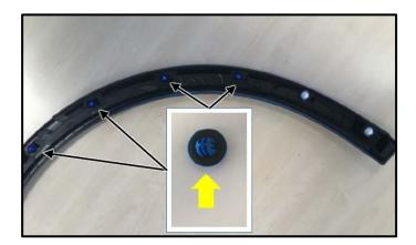
Verify that the black foam washers <arrow> are still installed on the remaining blue clips.
