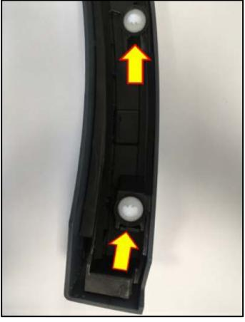
• Install the new white clips in the opposite direction of removal.
