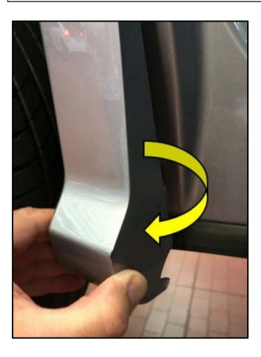
• Unclip wheel arch trim "cap" by turning and pulling simultaneously.
