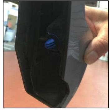
Carefully hold the wheel arch away from the vehicle.
