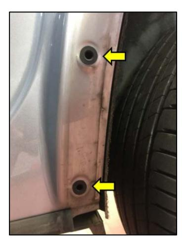
Install/replace the two lowest grommets <arrows>.
