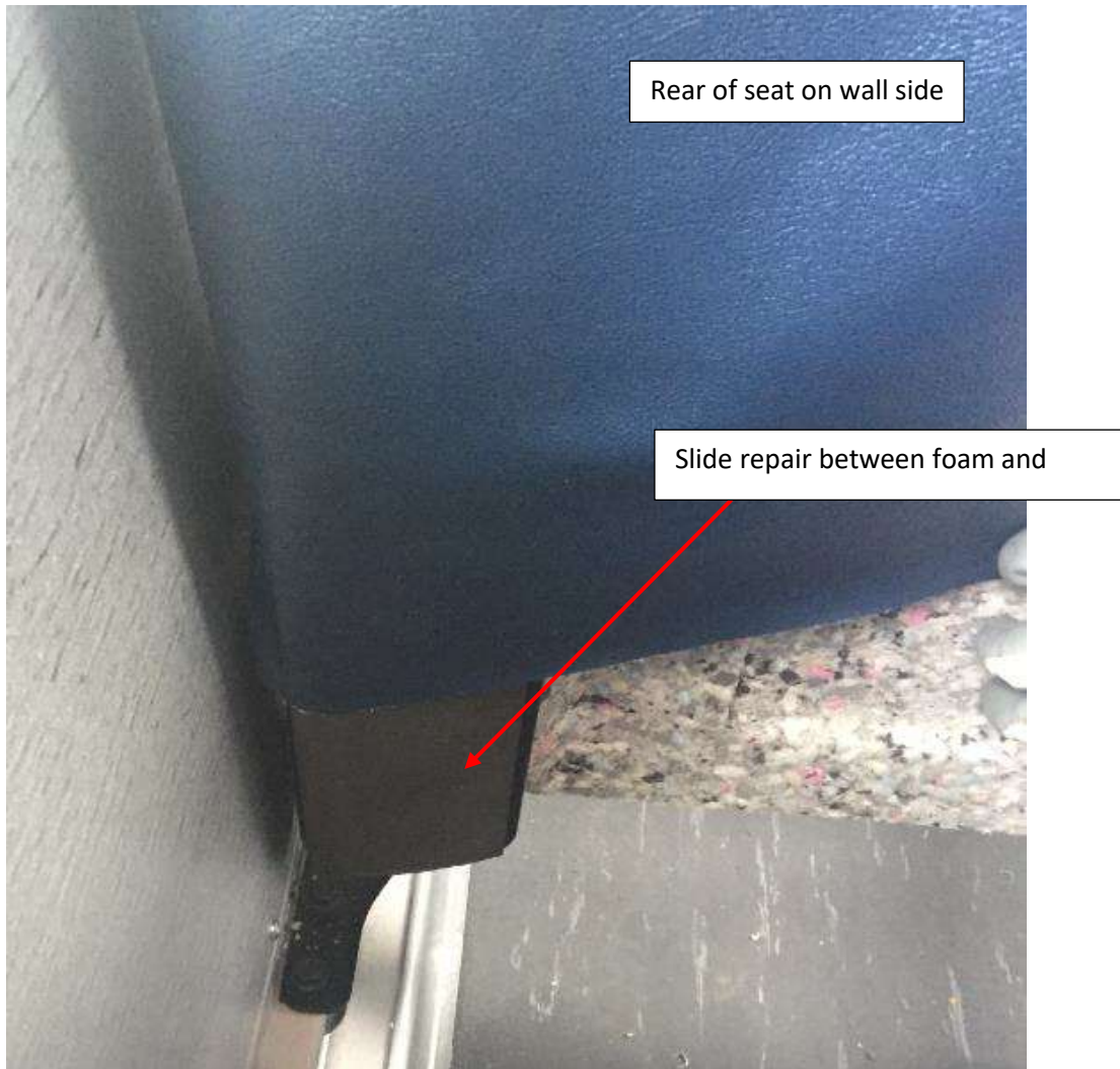
Figure 7: Seat shown with repair part being inserted
