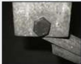
**STEP 3:** Remove the spring eye bolt and discard.
