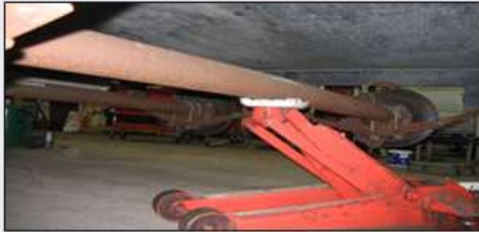
**STEP 3:** Use the floor jack to support the forward axle, gently raise the axle to remove weight from the center equalizer.
