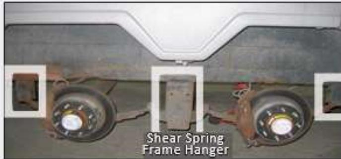
The center tower portion is the frame hanger for the MORryde LRE Shear spring, and the outside frame hangers are the positions for the front and rear leaf spring eyes. If your suspension assembly does not resemble this picture, please stop installation and contact MORryde for a review of your unit to determine the proper kit needed for installation on your trailer.
