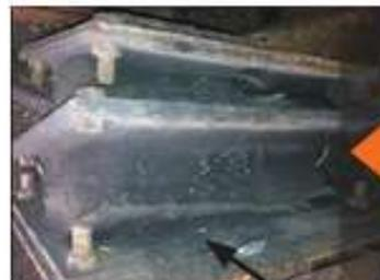
Tears exceed 3" long and  $\frac{3}{8}$ " deep, springs SHOULD be replaced.
