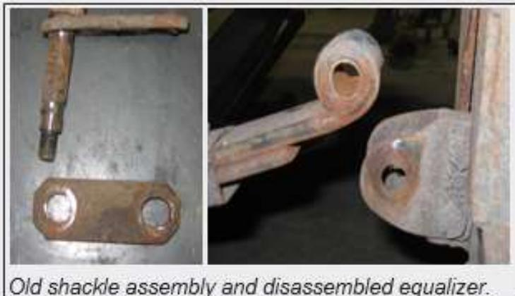
Old shackle assembly and disassembled equalizer.
