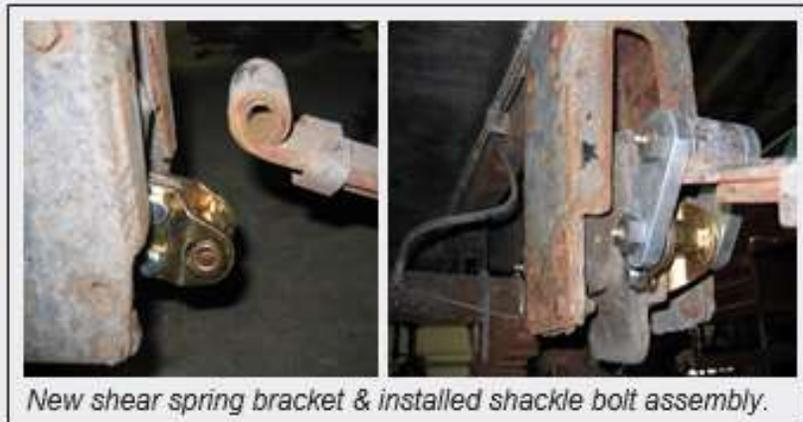
*New shear spring bracket & installed shackle bolt assembly.*
