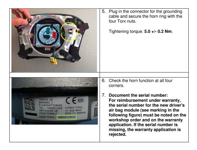
See repair instructions **REP 32 34 020** "Remove and install / replace air bag units" to complete installation.
