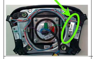
3. Place the horn contact plate on the new air bag module and plug in the connector.
