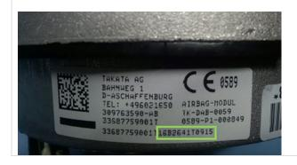
Note: Before installing the replacement part, the new air bag module's serial number must be documented by the technician on the repair order so it can also be entered into the warranty claim's comment section.
