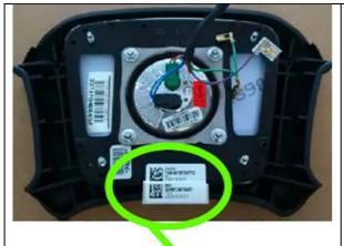
2. Prepare the new air bag module and pull off one of the two labels with the barcode and serial number of the air bag module. This must be stuck onto the horn ring after installation.
