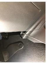
• CAREFULLY unsnap the trim, disconnect the switch harness connectors and set the panel aside.
