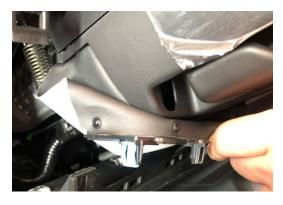
• Remove the 2-10mm hex nuts securing the knee airbag module and set it aside on end as shown. **NOTE:** There is no need to disconnect the airbag harness connector from the module.
