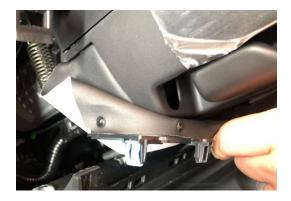
• Remove the 2-10mm hex nuts securing the knee airbag module and set it aside on end as shown. **NOTE:** There is no need to disconnect the airbag harness connector from the module.
