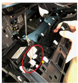
CAREFULLY release the fabric lower column cover trim from the top edge of the knee airbag module. There are 2 retaining clips (one on each end) and 2 alignment tabs in the middle.
