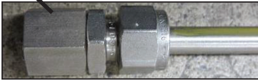
Figure 39: Reinstall the normal pin cap.
