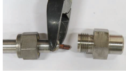
Figure 33: Wire from the LT130 being cut at the centering washer.
